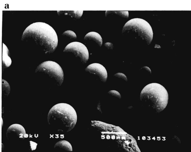
Figure 1. Scanning electron microscopy (SEM) micrograph of PVP-2%/MTO catalyst.
